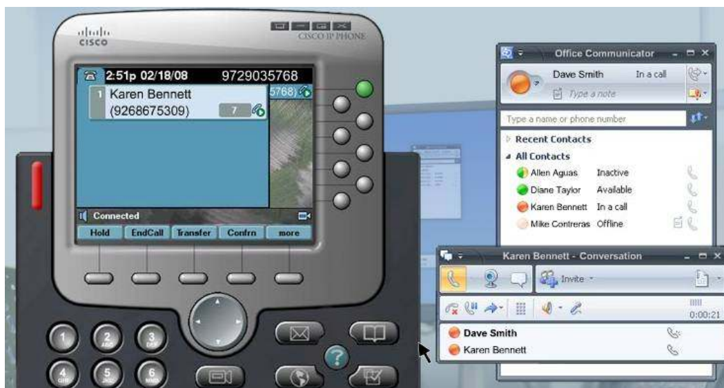
Figure 2. Click-to-Call Dialing and Third-Party Call Control of Cisco Unified IP Phones Using Microsoft Office Communicator 2007 and Cisco Unified Communications Manager
